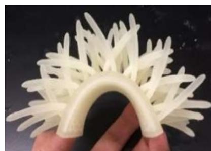
Preliminary lab prototype of UA's impact protection technology, which mimics hedgehog spines
